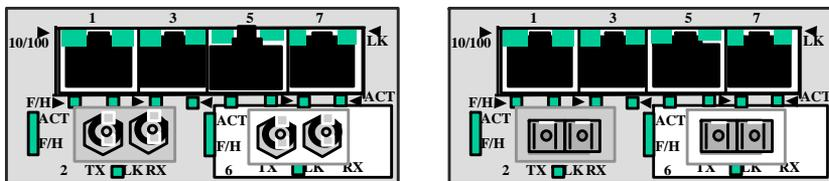
SC or single mode SC or Long Reach SC ports. For ports numbering, ports 1,3,5,7 are copper, ports 2 and 6 are fiber, ports 4 and 8 are not present.
