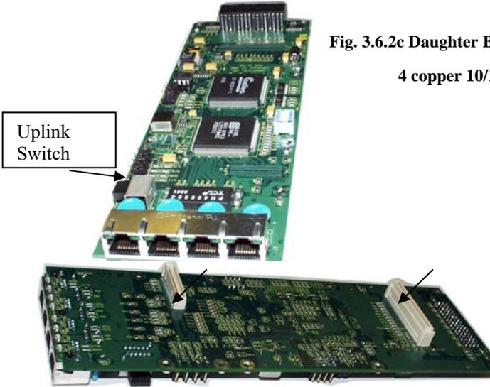
**Fig. 3.6.2c Daughter Board, top view of 4 copper 10/100 ports**
