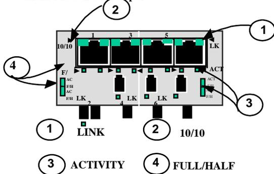
The Magnum 6KP8-45LC Module is a combo module with a combination of copper and Fiber (Small Form Factor) LC type ports. The small size of LC connectors allows an advantage of having more ports on one module. The
