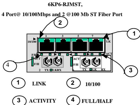
Each port has an Activity (ACT) LED indicating packets being received, a Link (LK) LED that indicates proper connectivity with the remote device when lit, and FDX/HDX LED to indicate full-duplex mode when lit (or half-duplex when off). The 10/100 LED indicates the speed, if the LED is ON 100Mbps if it is OFF 10Mbps.
