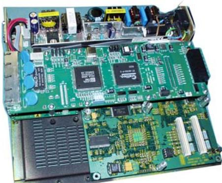
after successfully installing the 6KPM cards inside the Magnum 6K16-Series.
