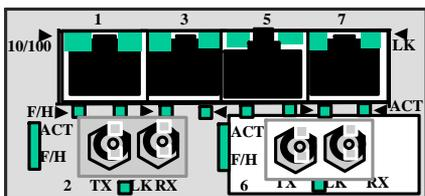
The Magnum Combo six-port modules are also available with 4@ MTRJ 100Mb mm SFF fiber and 2@10Mb fiber mm ST ports, and with 4@ RJ45 10/100 copper and 2@10Mb fiber mm ST ports. The
