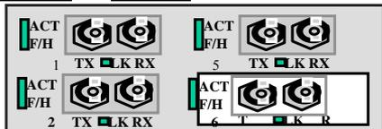
The 4-port @10Mb ST fiber modules behave the same as the 4@100Mb ST fiber modules except for the 10Mb speed. For ports numbering, ports 1, 2, 5, 6 are present, ports 3, 4, 7, 8 are not present. There is also a similar 100Mb fiber SC module.
