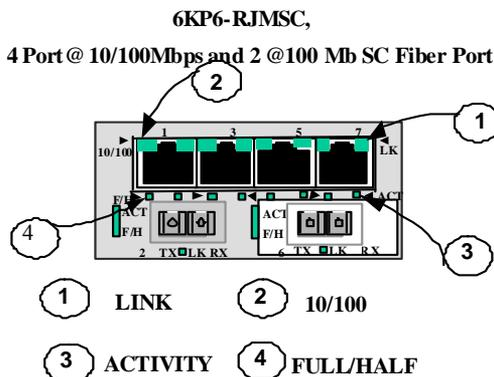
While the functionality of these two modules is essentially the same, the 6KP6-RJMSC is equipped with an SC-type "snap-in" connector instead of an ST-type.
