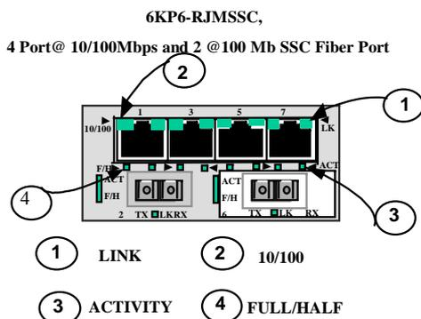
The 6KP6-RJSSC, when installed in a Magnum 6K16-Series Switch operates on copper at the 100m distance. The Fiber is single-mode and cable lengths can be as much as 25+ Km (see Power Budget, Section 4.5)
