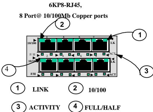
**Important Note:** The 10/100 RJ-45 ports are supported with Auto-negotiation and Auto-crossover (MDIX), which allow the RJ-45 ports to automatically Link with any RJ-45 device and eliminate the use of cross-over cable.
