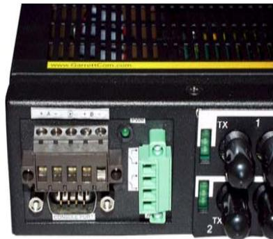
The second (bottom position) NC Alarm Contact is held close when there is power on the main board inside of the 6K16. This provides a "Hardware Alarm" because
