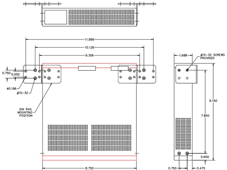
The unit can be mounted using the brackets turned outside (normal) or inside (if space is tight). Attach the mounting bracket either outside or inside as shown in the illustration above (dotted line shown for the brackets inside). The spacing for the mounting screws into the supporting wall or panel is a rectangle 11.89" x 7.85" center-to-center.
