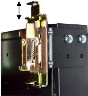
required two screws are included with the DIN-Rail brackets, and are no.10-32 X 3/8 PHIL. PAN w/star washer. The two heavy duty Din-Rail latches are designed as if that they can be manually accessed from the top when the 6K16V is installed on a DIN Rail.
