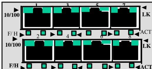
Using the 6K16-Series (MNS-6K) management software, the user may disable auto-negotiation and fix the desired operation of each RJ-45 port. User may select 10Mb or 100Mb speed and full- or half-duplex mode per-port as per user requirement. (See Magnum MNS-6K Software Manual for details info).
