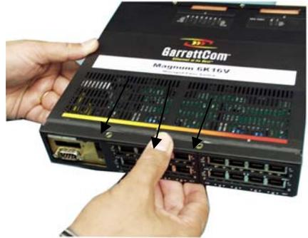
**Figure 3.6.1a: Removing the Front panel from the unit**
