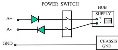
The manual power “On-Off” Switch (optional) is used for powering the unit on and off when it is placed into or taken out of service.
