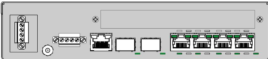
The 6KL-2GSFP 2-port Fiber Gigabit module provides two SFP open transceiver locations. Transceivers are available with both multi-mode 850nm (550m), 1310nm (2km), single-mode 1310nm (10km and 25km) and single-mode 1550nm (40km and 70km) fiber options. (see Sec. 1.2 of this manual for available part numbers)
