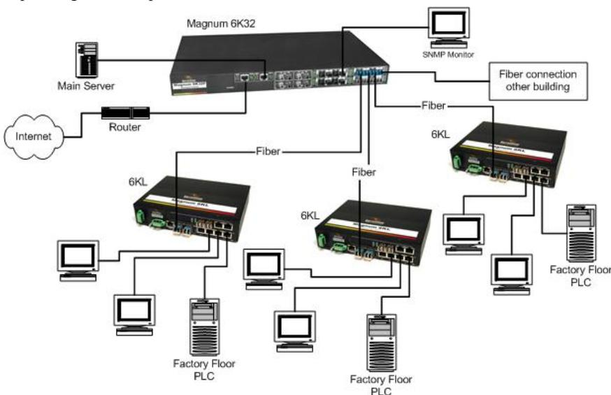
**Fig 2.5a The industrial factory floor application with Magnum 6KL**
