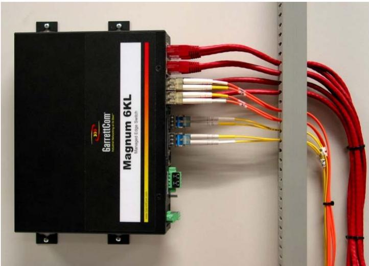
**Fig 3.3.1c** Typical Panel / Wall mounting of the 6KL Switch (position 2 shown)
