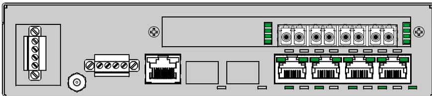
The 6KL4-4MLC 4-port Fiber module provides four 100Mb Multimode LC Fiber ports.
