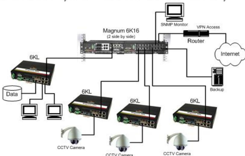
**Fig 2.5c** Magnum 6KL deployed in a video security CCTV application for monitoring and securing the premises
