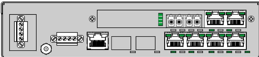
The 6KL4-2MLC2RJ 4-port Fiber / Copper module provides two 100Mb Multimode LC Fiber ports and two 10/100Mb switched RJ-45 ports.
