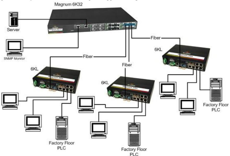
**Fig 2.5b Magnum 6KL equipped with S-Ring in redundant ring solution**
