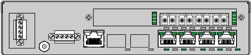
The 6KL4-2SL2MLC 4-port Fiber module provides two 100Mb Singlemode LC Fiber ports and two 100Mb Multimode LC Fiber ports.
