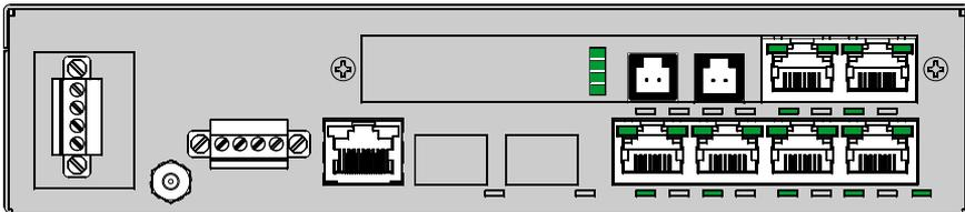
The 6KL4-2MT2RJ 4-port Fiber / Copper module provides two 100Mb Multimode MTRJ Fiber ports and two 10/100Mb switched RJ-45 ports.
