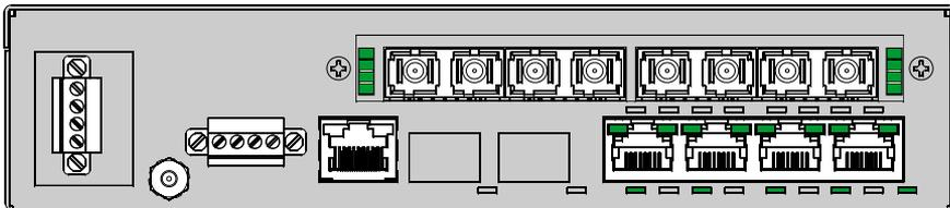
The 6KL4-4MSC (shown) 4-port Fiber module provides four 100Mb Multimode SC Fiber ports. This option utilizes a SC-type “push-pull” fiber optic connection.
