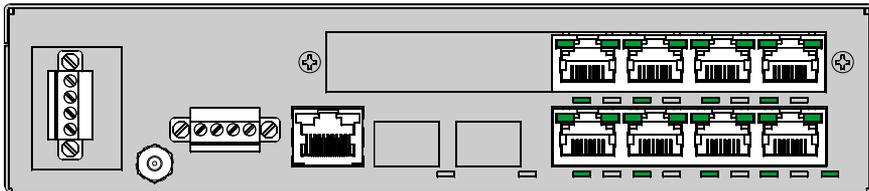
The 6KL4-RJ45 4-port Copper module provides four 10/100Mb switched RJ-45 ports. The 10/100Mb switched ports normally (as a default setting) are independently N-way auto-negotiating and auto-crossover (MDIX) for operation at 10 or 100Mb speed in full- or half-duplex mode. (i.e., each independently selects a mode and speed to match the device at the other end of the twisted pair cable).
