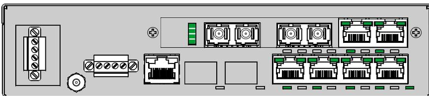
The 6KL4-2MSC2RJ (shown) 4-port Fiber/Copper module provides two 100Mb Multimode SC Fiber ports and two 10/100Mb switched RJ45 ports. This option utilizes a SC-type “push-pull” fiber optic connection.
