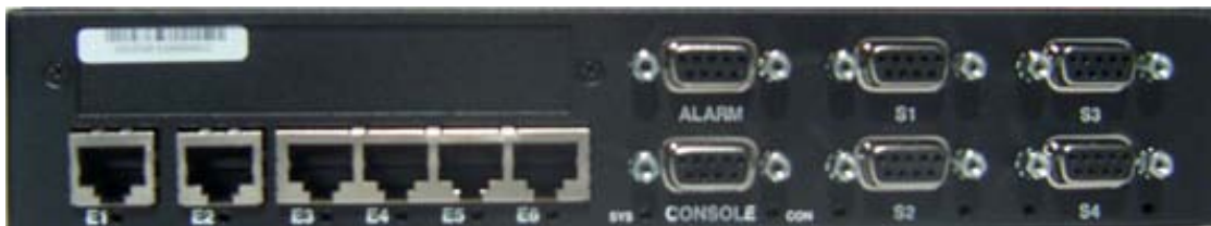
Figure 1-1(a) - Front View of DX940 (without the WAN port). This view shows the optional Gigabit Ethernet ports E1, E2; 10/100 Ethernet port E3 to E6 and optional serial ports S1 to S4.
